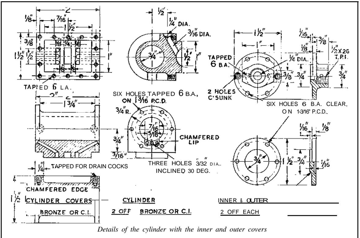
Details of the cylinder with the inner and outer covers
