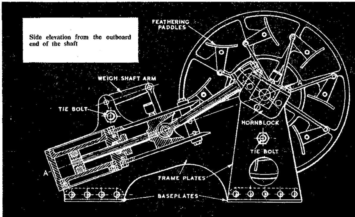
In the structure of the engine, steel plates are used, mainly in the interests of simplicity. Although most large paddle engines employed more or less complex structural castings, often incorporating a surface condenser and other working parts, the use of plate frames was by no means unknown in the smaller and less elaborately-equipped engines.
