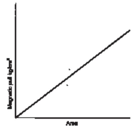
(ii) The proportional relationship between magnetic pull and workpiece area.
