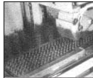
**7. For one off machining** of small, thin components a Fine Pole Chuck should be used. The component being placed across a brass lamination to achieve maximum hold.
