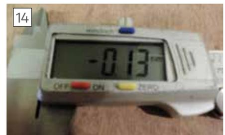
14 *The Workzone caliper was most affected by changing temperatures, drifting about 0.007mm per degree, enough to cause material errors in the average workshop.*
