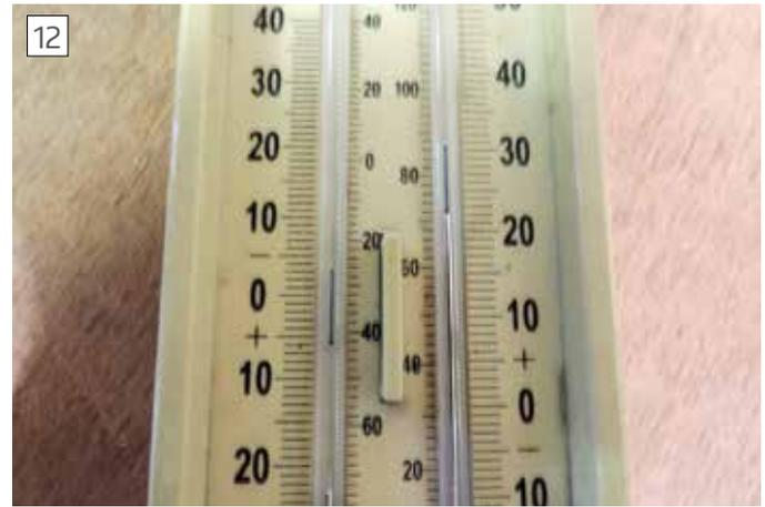
12 *A max-min thermometer was used for the temperature stability test.*
