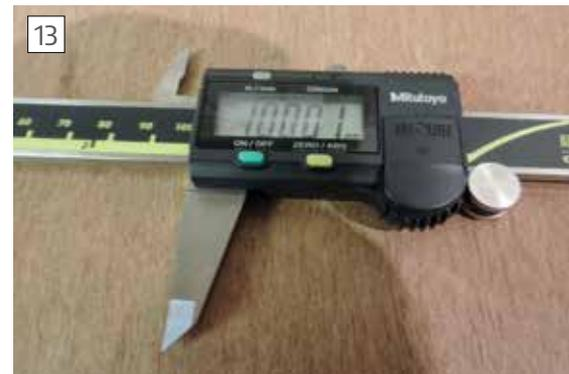
13 *A seventeen-degree temperature change did not affect the Mitutoyo's reading – the M&W caliper was also rock solid.*
