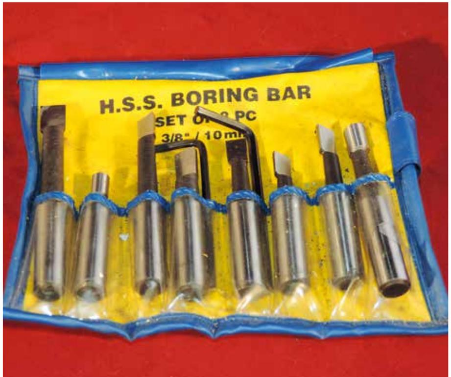
*A set of boring tools, together with allen keys to fit the boring head.*
