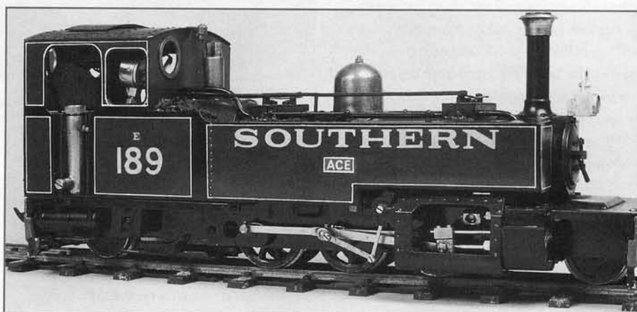
This 16mm narrow gauge locomotive is modelled on the Lynton & Barnstaple Railway's 2-6-2 "Yeo" and runs on 32mm gauge track. It has been very successfully converted to coal firing by Shawe Steam Services.
