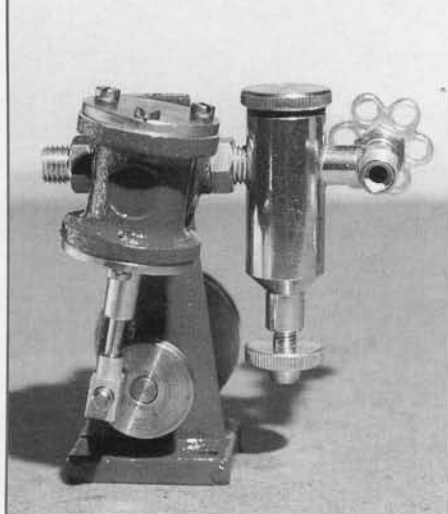
The complete engine assembly is shown here with the lubricator and stop valve and the engine exhaust union in place. The engine could be used in this condition to power many different sorts of model e.g. small railway locomotives or steam trams etc.
