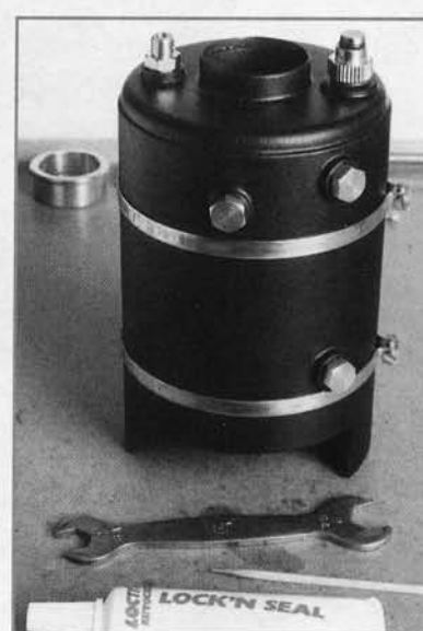
The boiler is shown here with all the fittings in place. Blanking plugs are used in bushes where optional accessories may be fitted.
