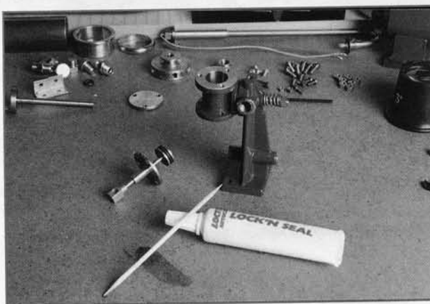
Above: First stage - cylinder & trunnion pin assembled and held in column while sealant cures; big end fitted to piston rod with bottom cylinder cover in place. Below: Securing the cylinder cover in place with the screws provided.
