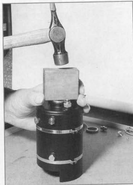
Left: Carefully pree the chimney coupler in place in the boiler spigot by hand and then tap it down using a hammer and wood block. Keep checking that it goes in square. Right: You may need to turn the block on edge to clear the safety valve and union, if already fitted, (see note in text about this operation) in order to seat the coupler right down on the spigot.
