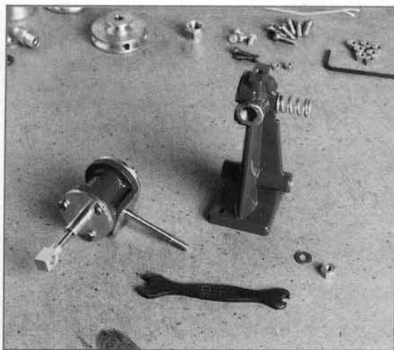
Having completed the cylinder assembly - with piston in place and end covers fitted - it is now ready to attach to the column.
