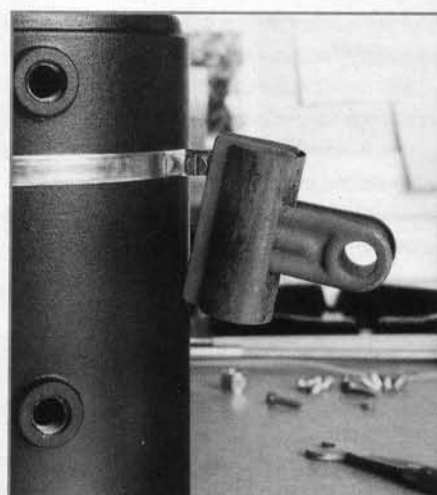
First job on the boiler is to fit the boiler bands. I found the use of a small Bulldog clip helped to hold the ends together when fitting the bolt and nut.
