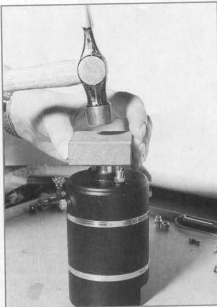
Left: Carefully pree the chimney coupler in place in the boiler spigot by hand and then tap it down using a hammer and wood block. Keep checking that it goes in square. Right: You may need to turn the block on edge to clear the safety valve and union, if already fitted, (see note in text about this operation) in order to seat the coupler right down on the spigot.
