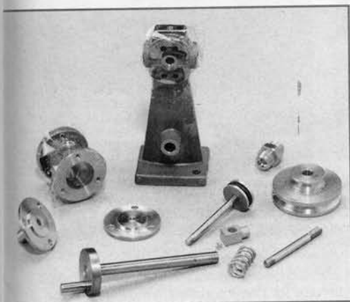
Top: This view shows the working set-up on a board on the desk. Above: The fully machined engine parts as supplied - cylinder & covers, column, piston and rod, flywheel and crankshaft.
