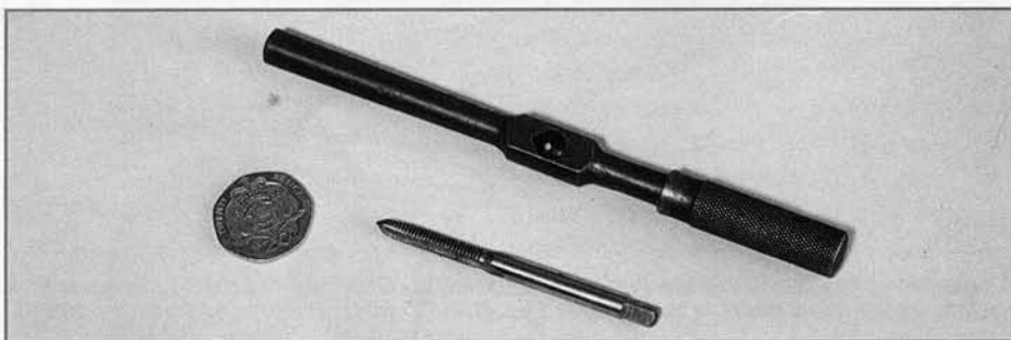
This photo shows a flat type of tap wrench. Be careful to exert pressure evenly on both ends otherwise you will risk breaking the tap.
