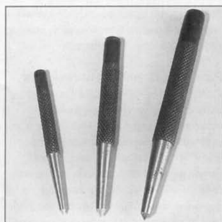
set of three sizes of centre punch made by Eclipse tools. (See close-up photo below for how to centre punch accurately).
