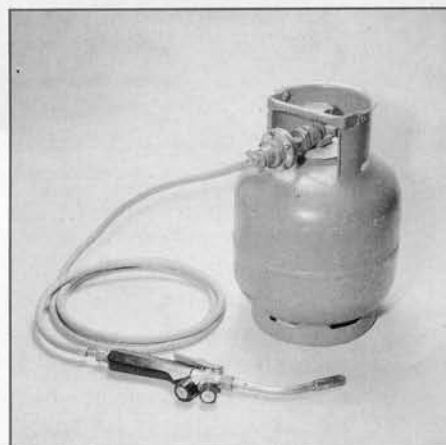
A convenient size of gas bottle for smaller work is shown here with a hose and gas torch fitted.
