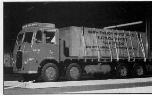
Gerald Webb won a Gold Medal at the recent Model Engineer Exhibition at Olympia for his 1/12th scale model of a 1947 Leyland Octopus 22 ton 8 wheel lorry. This is a fully engineered model built on the same principles as its full size prototype.
