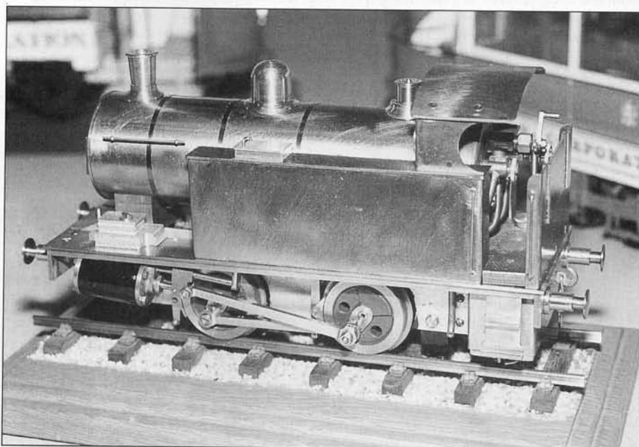
LBSC's "Juliet" design is an ideal beginner's loco which is quite easy to build. This unpainted example seen at the recent Model Engineer Exhibition is built to Gauge '1' standards to run on 45mm (1 3/4") gauge track.
