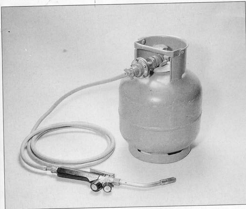
A small propane gas cylinder with regulator and non-return valve, high pressure hose and Sievert torch.
