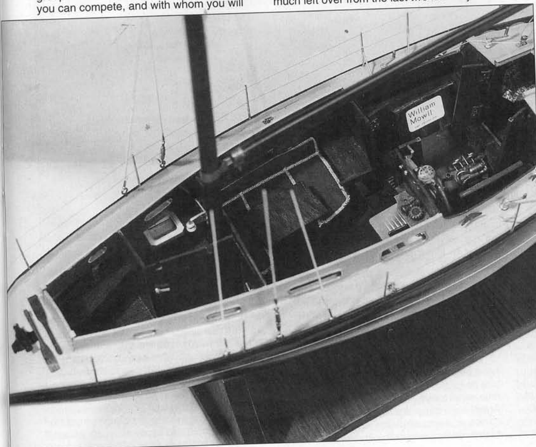
My first scratchbuilt model. A Camper & Nicholson 38' ketch rigged yacht, made from dockyard plans in 1976 at a scale of 1:16. Constructed from timber, it includes several items of interest to the scratch-builder; the forward head basin is made from an old razor blade dispenser; the head itself (not visible) from a hinged Smartie tube cap. The engine is a 'Tick Tack' sweet box, overlaid with electrical condensers; and the working steering gear uses the machine head worm gear from a guitar tuner, ratio approx. 50:1. Whereas it is not a true working model, the keel is ballasted so that she is quite at home in the water.
