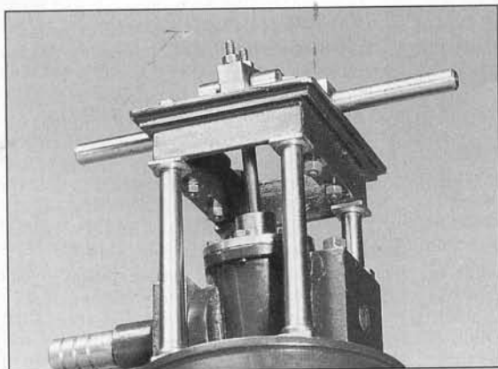
This underside view shows the fixing nuts for the main bearing bolts.
