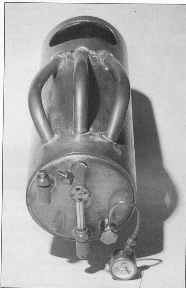
An end view of the boiler showing arrangement of water tubes and backhead.
