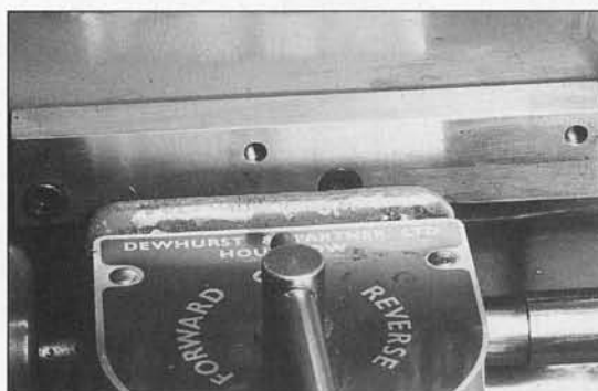
The raising block fitted in position behind the drum reversing switch.
