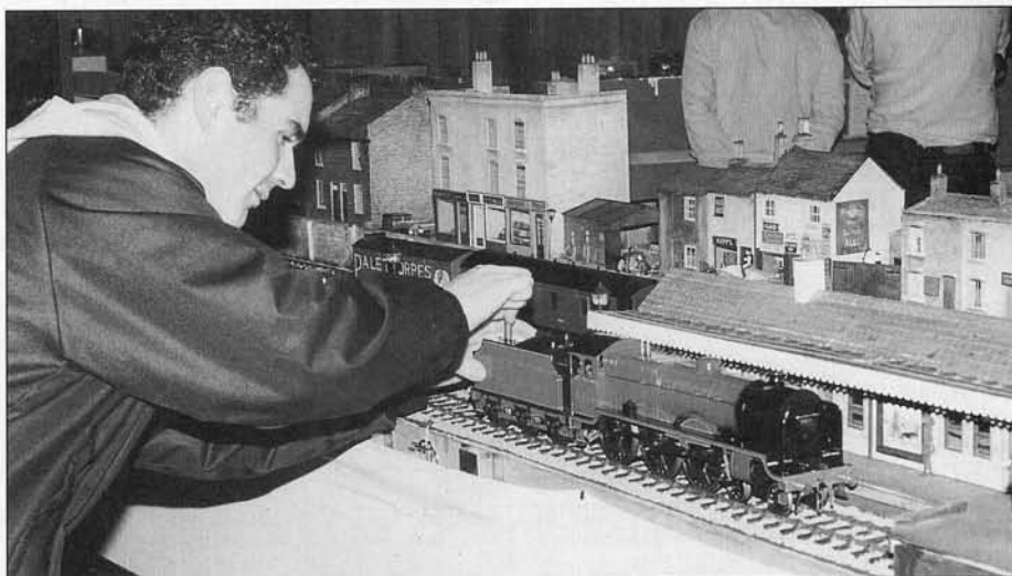
Using the tender hand pump to top up the boiler water level on a live steam, spirit fired Gauge '1' LMS Patriot 4-6-0 Lady Godiva.
