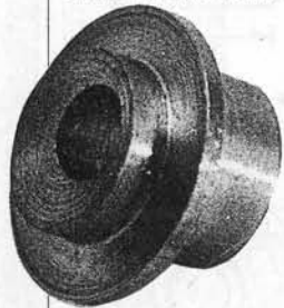
Above, close-up of the finished eccentric.
