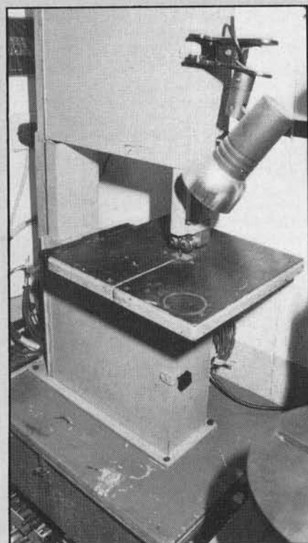
Charlie's homemade band saw is constructed entirely of angle iron and sheet metal and the wheels which convey the blade are from wood with inverted rubber-toothed belts set in the periphery.
