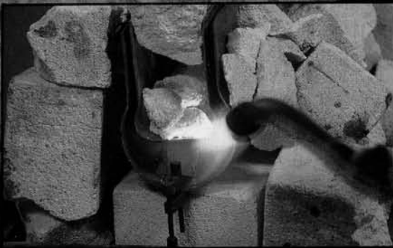
The crown stays are soldered to the outer firebox. Without the preheat, temperature raising of the joints would have taken too long.
