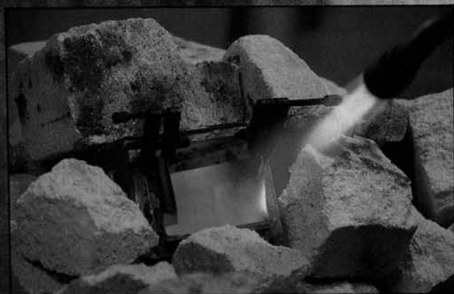
The inner stays are silver soldered with Easyflo 2. Leaving the firebox rear off helps with this operation, but makes it more difficult later on. Previously soldered joints are protected here by a stainless steel strip. Below and right: silver soldering the foundation ring into position. If the backhead and rear firebox plate have been left in place, as here, the foundation ring can be done in one go.
