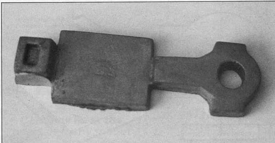
Castings are sometimes produced in 'sticks' which saves waste at the foundry. Here a slide valve, steam chest cover and eccentric strap have been cast as a single piece.
