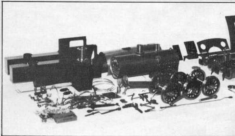
Above, the frames and buffer beam of a model Hunslet locomotive built by the author. The frames represent a cutting and filing exercise of no great complexity while the buffer beam involves a spot of simple drilling and riveting.
