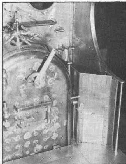
The rear of a boiler (backhead) on a model currently under construction by Bob Moore.
