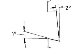
ENLARGED DETAIL OF SLOT WITH ANGLES SHOWN EXAGGERATED FOR CLARITY SLOT ANGLES TO MATCH STANDARD TOOLS.
