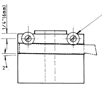
PARTING TOOL SECURED WITH TWO W 1/2"(12mm)DIA ×3/32"(2.5mm)THICK C/ACCEPT 25 A. (4m) C/SUNK SCREWS.
