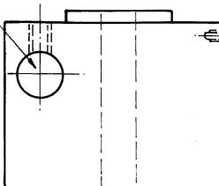
THREE HOLES TAPPED 1/4'(6mm) FOR SCREWS TO SECURE BORING BAR.
