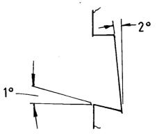
ENLARGED DETAIL OF SLOT WITH ANGLES SHOWN EXAGGIFOR CLARITY SLOT ANGLES STANDARD TOOLS.
