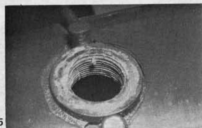
35 Large bush silver soldered in boiler, for safety valve.
