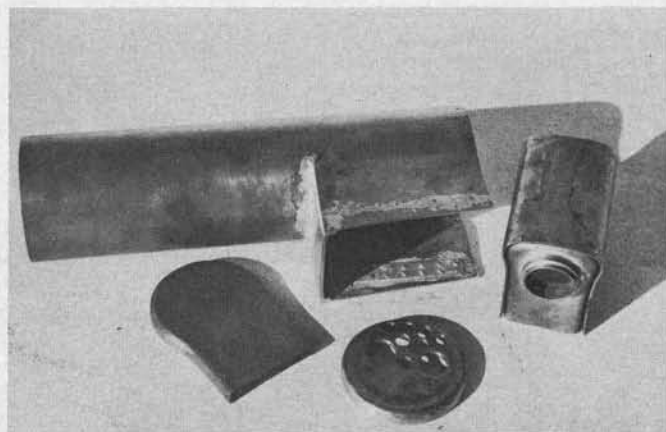
14 Components of a small round top boiler.
