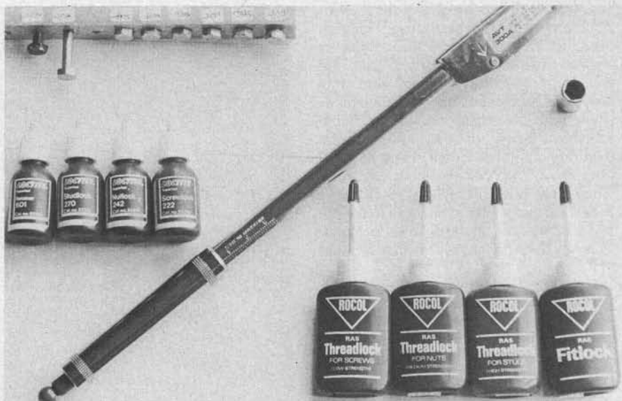
The author tested this range of anaerobic adhesives, evaluating the bond strength, using a torque wrench
