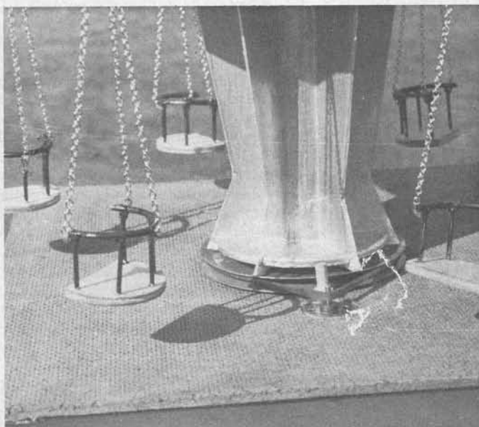
Rubber band drive and chain-hung seats
