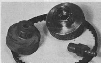
Crankshaft adapter, flywheel with clutch shoes fitted and drive belt
