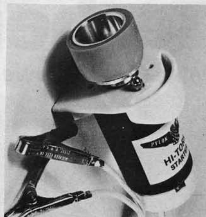
Electric hand-starter with rubber ring as provided. A hard rubber is recommended as soon as the original is worn out
