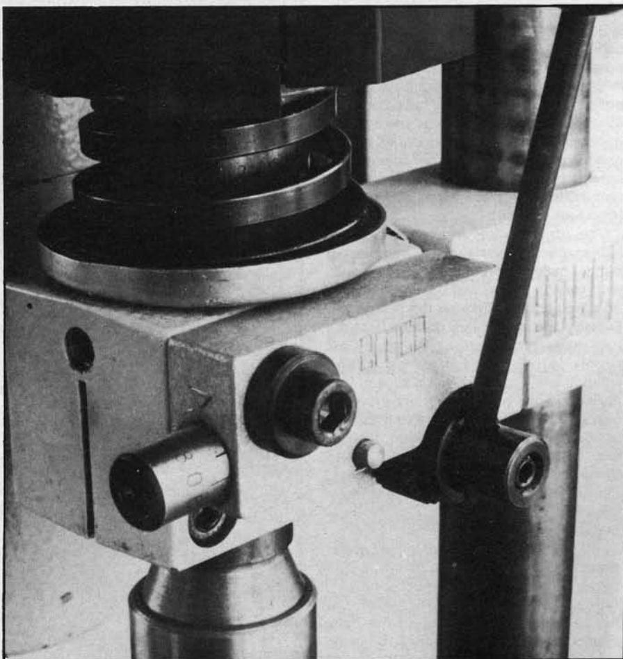
Vertical fine-feed attachment. An Allen key is used to advance the calibrated mechanism
