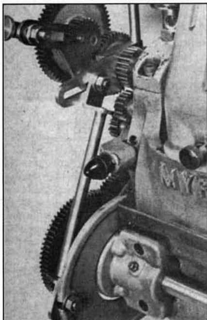
The compound dividing attachment in use on the lathe. The big index wheel is 60 t, keyed to the 25, gearing with 45 wheel on the mandrel. Indexing round by "threes" gives 36 divisions.
