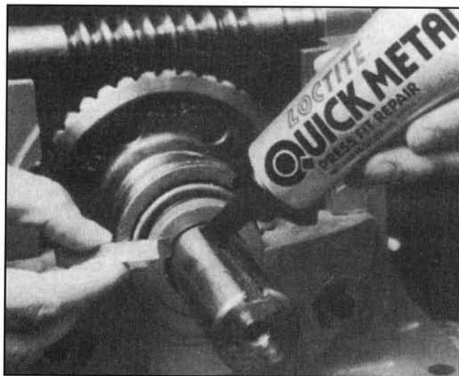
Loctite Quick Metal was used to take up backlash in this keyway.
