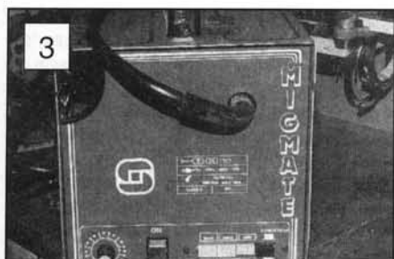
3: The front panel of the welder used, the black button is 'range'. White buttons are voltage settings.
