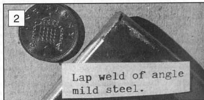
2: A lap weld on two pieces of 1mm mild steel angle after dressing.
