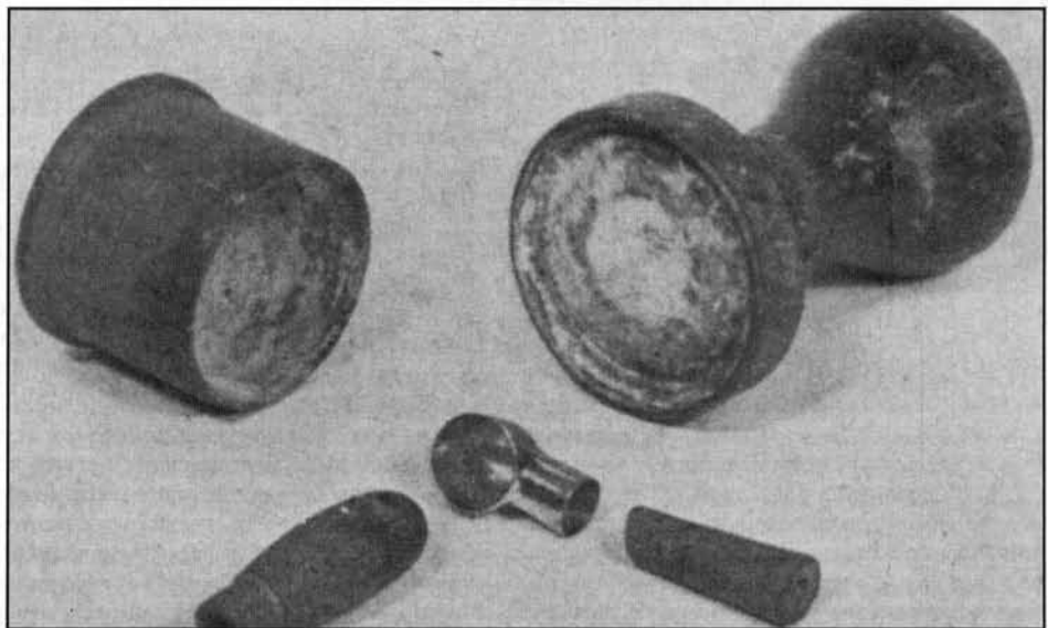
The open-ended ring and pressure pad, also wooden cores used in making the pattern for the ship's ventilator seen in centre.
