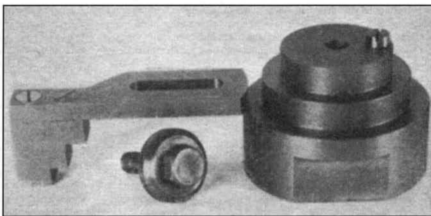
Fig. 6b The bending block dismantled, showing the component parts.
