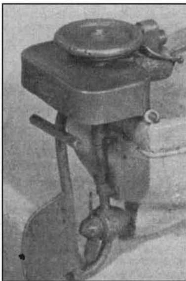
A model outboard motor cast in one piece.
