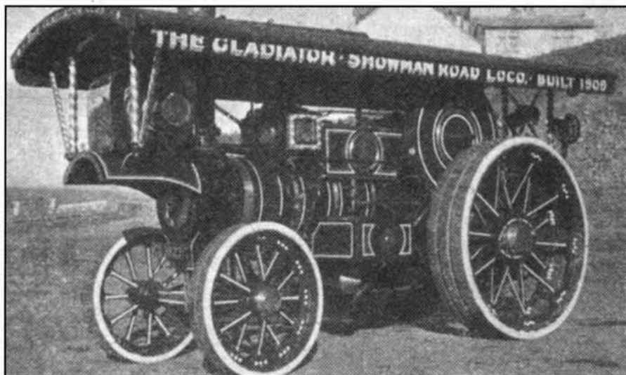
Three-quarter near side view, showing flywheel, worm drive for steering gear and copper top on chimney.
