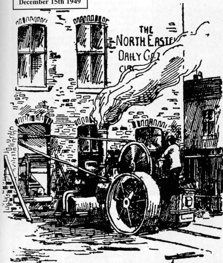
Mr. H. G. Greg, of Styal, Cheshire, has solved the transport problem by means of a miniature traction engine, which with a couple of bottles of water carried on a trailer and a bucket of coal, will run for many miles. It can haul half a ton and climb steep hills, and a year's tax costs only 5/- [25p!].
