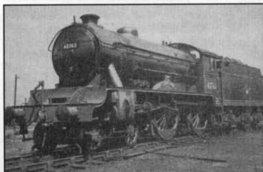
THE FITZWILLIAM, No.62763, the only member of the class fitted with Reidinger rotary valve gear.
