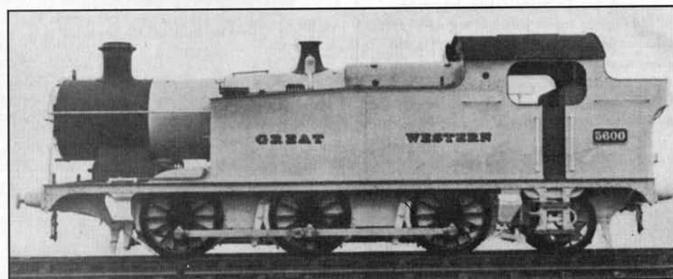
0-6-2 Tank Engine for heavy Coal Traffic, G.W.R.
