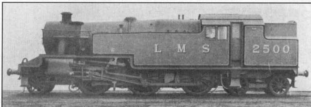
New 3-cylinder 2-6-4 Tank Engine, L.M.S.R.
