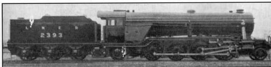
Profile of the L.N.E.R. "Mikado" Locomotive.
