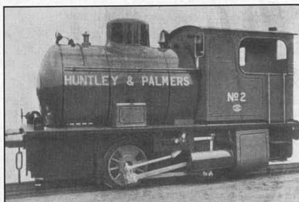
The Bagnall fireless locomotive for an industrial railway.
