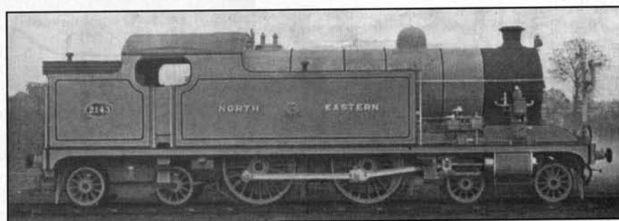
NEW TYPE OF TANK ENGINE, WITH THREE SINGLE-EXPANSION CYLINDERS: N.E.R.
