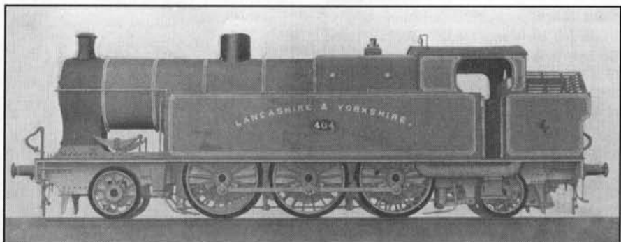
FIG.22—HEAVY 2-6-2 TYPE TANK ENGINE, LANCASHIRE & YORKSHIRE RAILWAY.
