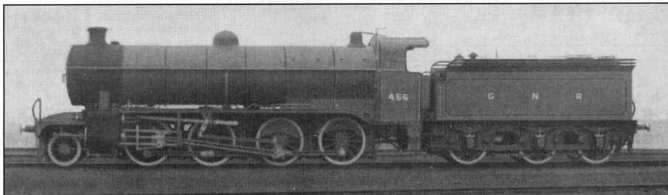
NEW 2-8-0 TYPE MINERAL LOCOMOTIVE: GREAT NORTHERN RAILWAY.
