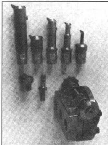
Some of the components of the boring head showing the tools used.
