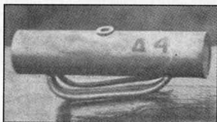
No. 4 boiler developed a small steam leak at 600 p.s.t., but otherwise it proved sound.
