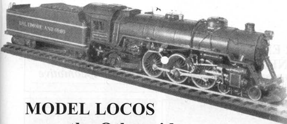
3/4 in. scale President Washington, Baltimore & Ohio Railroad, first built 1927. Cylinders 1 1/8 in. x 1 3/4 in. stroke; wheels 5 in. dia.; boiler barrel 5 in. dia.; weight with tender 140 lbs.
