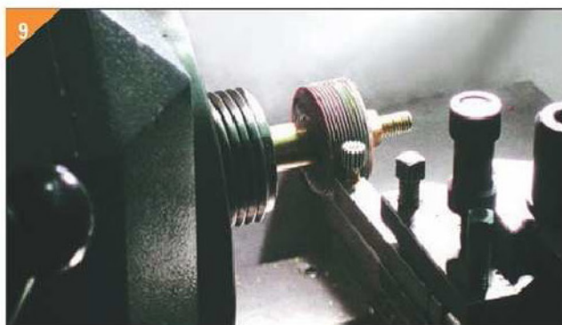
9. Set-up for polishing pinions.
