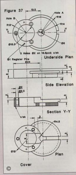
Using a slot drill mill out the recess down to 4mm. Leave the width of the recess slightly undersize. The cover is best finally fitted with the aid of a file. Drill and tap the two holes for securing the cover to the lifting tube. With the cover fitted in place, the ball entrance in the lifting tube can now be cut out.
