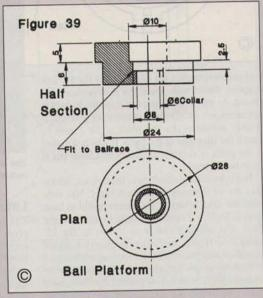
diameter section slightly overlength. The top of the platform has to be flush with the bottom of the entrance track bracket. Slide the platform into the lifting tube and press it firmly down against the shoulder in the tube. Mark with a scriber the bottom of the ball entrance. Remove the platform and face to its final length.
