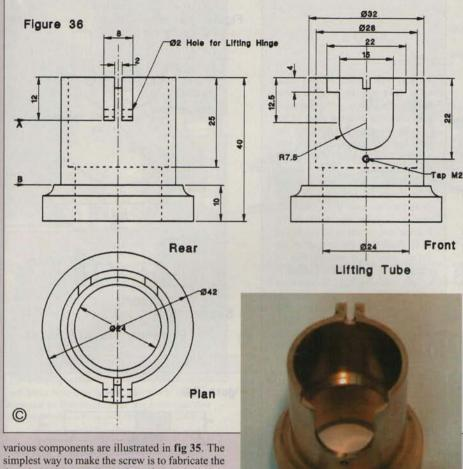
The lifting tube is machined from solid brass, including the hinge lugs, evident in this view.
