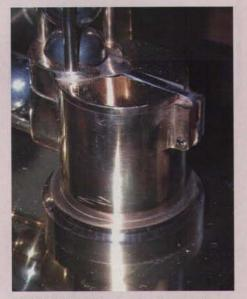
The finished ball lift mechanism showing the lifting tube, cover and entrance bracket. The non-return catch, to be described in a future article in this series, is also shown.
