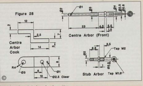
Insert the register pin in the cock and reposition the cock using the register pin to locate it. Check that the 3mm dia, rod still turns easily, clamp in position and drill and tap the 2.5mm dia. hole for the retaining screw. The aluminium bronze bush can now be made and fitted in the cock. Insert the ball race and the arbor and fit the cock in place. The arbor should spin freely with a small amount of end shake.
