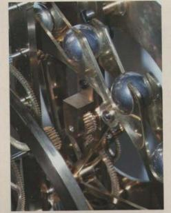
The centre arbor cock in position in the clock together with the respective wheels and pinions.
