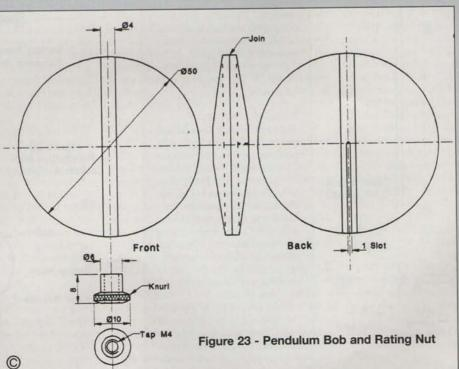
Face the end of the bar and part off a disc 7mm thick. Face the end again and part off a second disc. Clamp the two faced sides of the discs together in the vice on the milling machine. Using the centring microscope, position the axis of the milling machine spindle on the join and a line passing through the centre of the two discs as shown in fig 23. Drill and ream the 4mm dia. hole. Separate the discs and, using a 1mm milling cutter, cut the groove for the peg in
