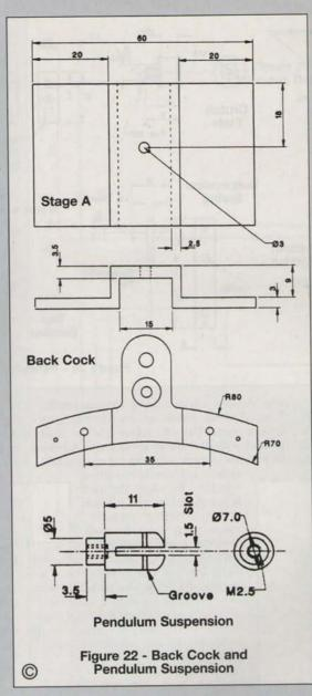
that the scribed lines are still correct. The cock can now be finished off using a piercing saw and files, referring to fig 22 as a guide for the shape. When the cock is finally pro-filed, the recess for the end cap can be drilled using the 8mm dia. counterbore, and the end cap fitted in place. The hole for the pendulum support is drilled 8mm vertically above the pivot hole in the cock.
