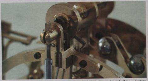
Some of the items referred to in the accompanying text are visible in this photograph. Note particularly the pallet arbor end cap, back cock, pendulum support and pendulum suspension spring.
