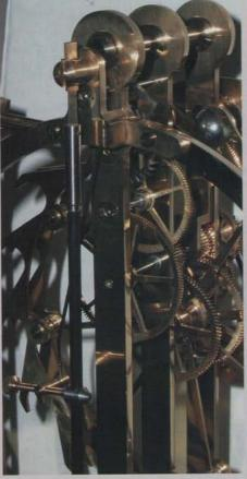
the carbon fibre pendulum rod and pendulum crutch assembly.
