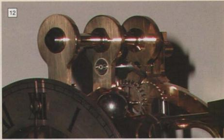
using the 8mm dia. counterbore. The recesses in the middle bar should be 1.5mm deep and those in the back plate 2mm deep.
