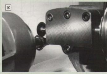
The method used by the author to correct the escape wheel geometry by means of a small carborundum cutting disc.
