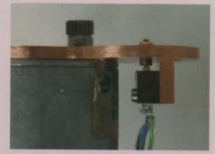
The micro switch and operating plunger mounted on the Archimedes screw drive motor mounting plate.
