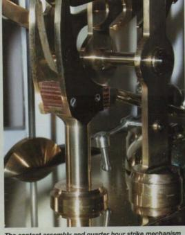
The contact assembly and quarter hour strike mechanism attached to the front time bar.
