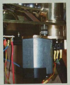
The Buhler 12V motor and its mounting as devised to drive the Archimedes screw and described by the Author for his prototype clock.
