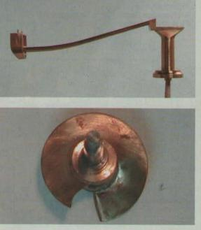
overall height of the vertical and delivery track should be such that the balls roll smoothly from the track onto the wheel. The vertical track rods were initially made a little overlength; these will have to be reduced in length to make the delivery from track to wheel smooth.
