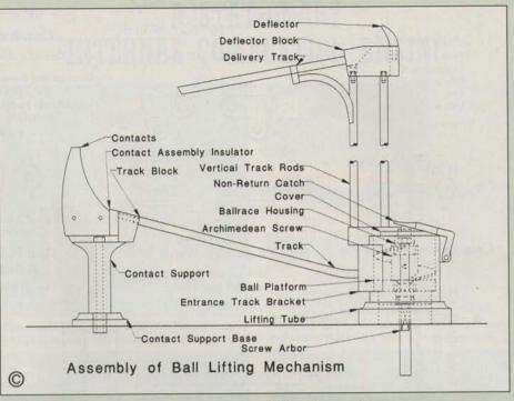
screw must be just below the surface of the shaft or it will foul the balls as the shaft turns.
