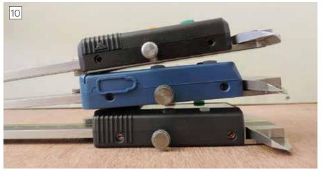
The three calipers all have reasonably sized gib screws, making adjustment easier.
