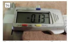
The Workzone caliper was most affected by changing temperatures, drifting about 0.007mm per degree, enough to cause material errors in the average workshop.
