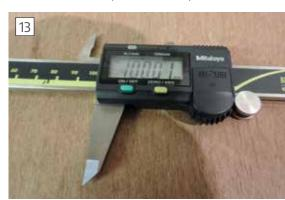
A seventeen-degree temperature change did not affect the Mitutoyo's reading – the M&W caliper was also rock solid.
