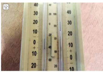
A max-min thermometer was used for the temperature stability test.
