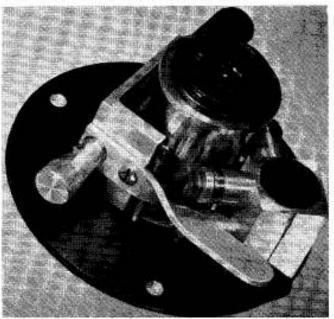
The focusing shaft is mounted on a hinged bracket which is made from pieces of aluminium alloy angle, and the bearings may be ball races, but if the mount is in brass, reamed holes to accept the diameter of the shaft with no slack will be sufficient. The shaft should not be greater than 6 mm. diameter as larger diameters will mean a loss of fine focusing action. Plastic knobs on each end of the protruding shaft ends will retain the shaft in
