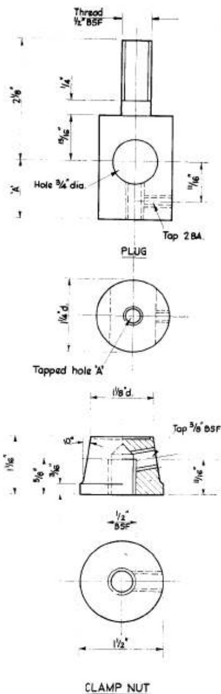
Note:- All dimensions are to suit lathe tool slot.
